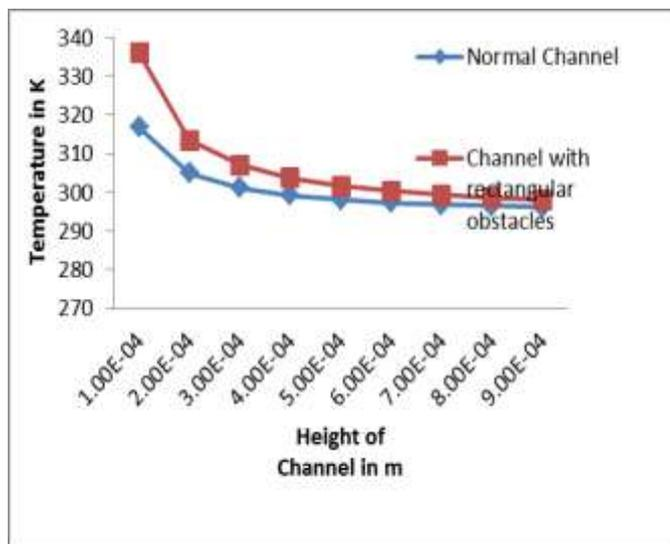
Figure 7. Effect of height of channel on temperature rise in fluid as water
