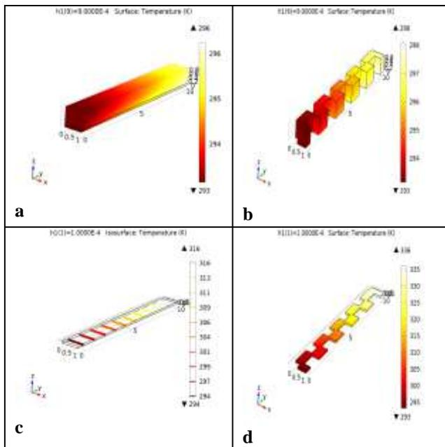
Figure 4. Temperature distribution in channel with and without obstacles
