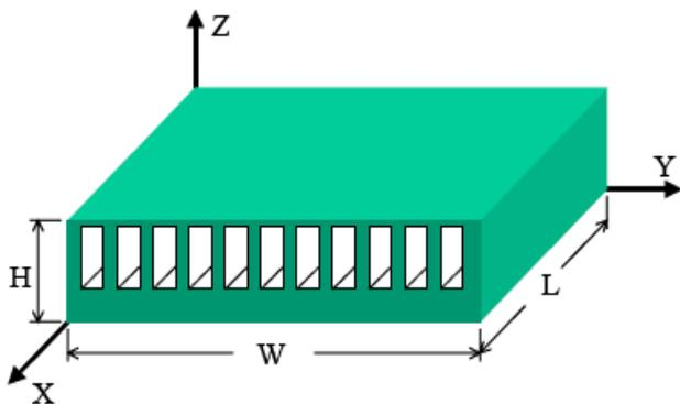
Fig 1: The schematic and overall dimensions of the micro-channel heat sink
