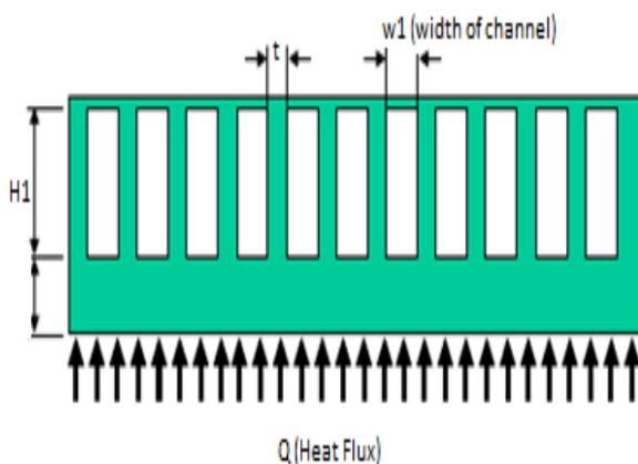
Fig 2 : Dimensions of the microchannel heat sink (The drawing is not to scale)
