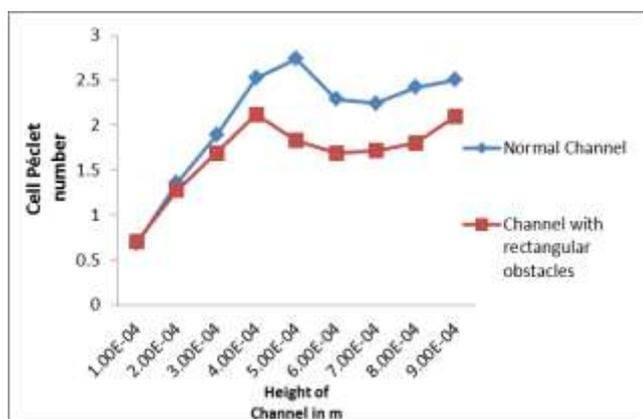
Figure 8. Effect of height of channel on cell Peclet number
