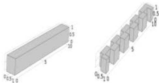
Micro channel without obstacle      Micro-channel with rectangular shape obstacles
