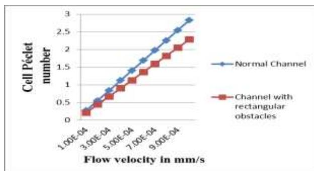
Figure 6. Effect of fluid flow velocity on cell Peclet number
