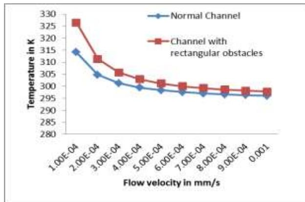
Figure 5. Effect of fluid flow velocity on temperature rise in fluid as water
