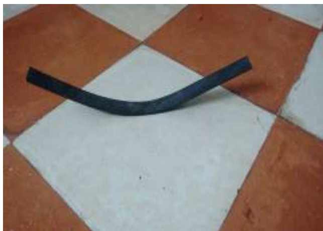
Fig. 3: 6mm ms sheet bend by machine
