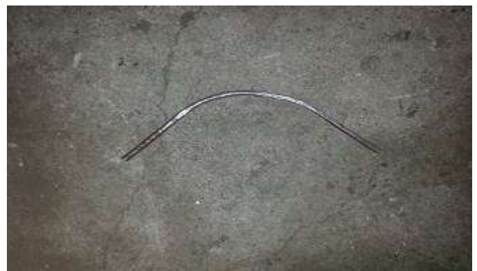
Fig. 7: Circular Pipe Bend
