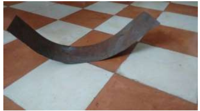
Fig. 4: 4mm ms sheet strip bend by machine
