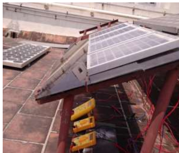
Figure 1: Experimental setup of the cement dust Solar module kept at 20°
