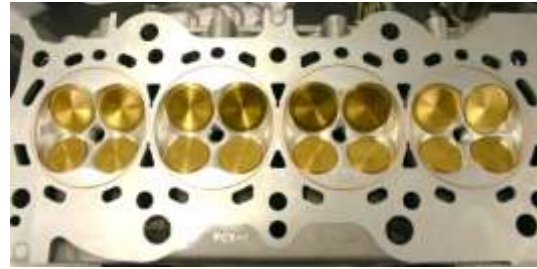
Fig. 2. Ceramic coating applied to inlet and exhaust valves.
